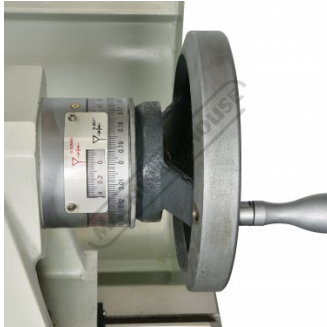
Tailstock Dial With Dual Graduations
