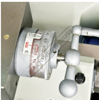
Compound Slide Dial with Dual Graduations
