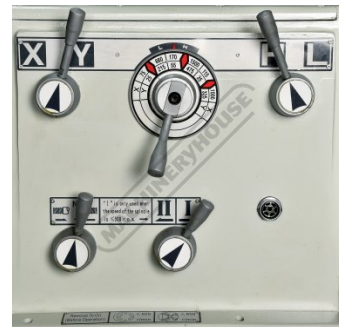
Speed Selection Levers and Feed Levers
