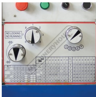
Gearbox And Thread And Feed Charts
