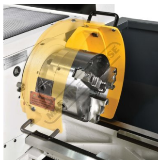
Chuck Guard with Safety Micro Switch
