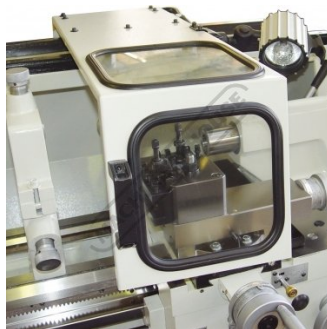
Sliding toolpost guard deflects swarf into tray
