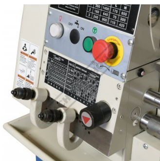
Feed Threading Levers and Control Panel
