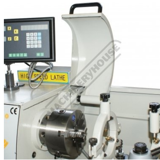
Chuck Guard with Micro Switch
