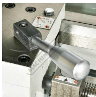
Longitudinal and Cross Feed Engagement
