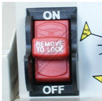
Safety Interlock Switch
