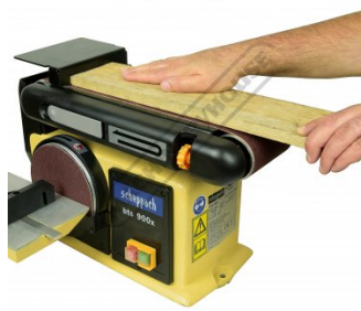
Shown Horizontal Flat Sanding
