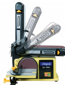
Horizontal to Vertical Linishing
