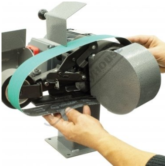
Remove and Replace Belt
