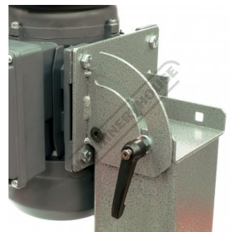
Head Tilt Hand Lever Lock
