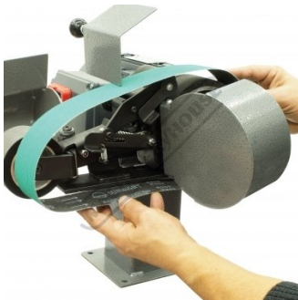
Remove and Replace Belt
