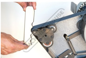
Small Wheel Selection for Notching & Contouring
