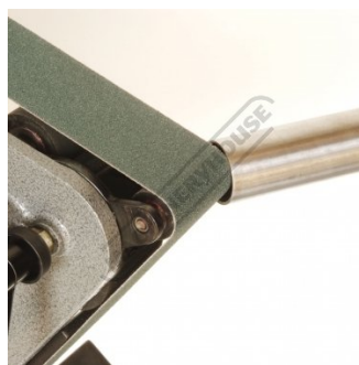
Internal Pipe Chamfering
