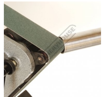
Internal Pipe Chamfering
