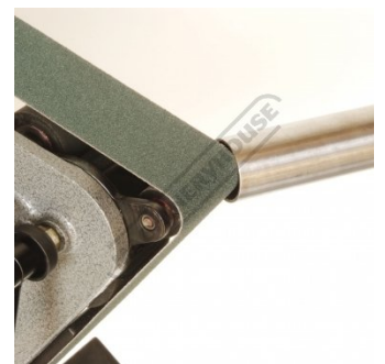
Internal Pipe Chamfering
