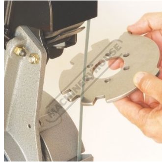
De burring & Finishing Irregular Shapes
