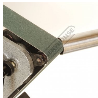
Internal Pipe Chamfering
