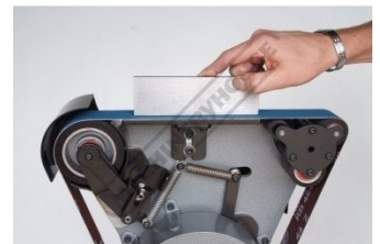
Flat Grinding on Platen
