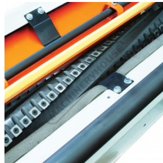
4 x Spiral Cutter Head with Carbide Inserts
