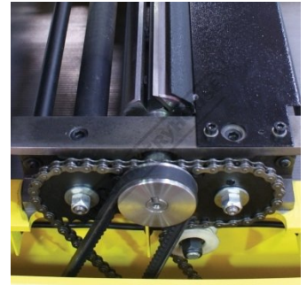
Chain Drive Feed Rollers
