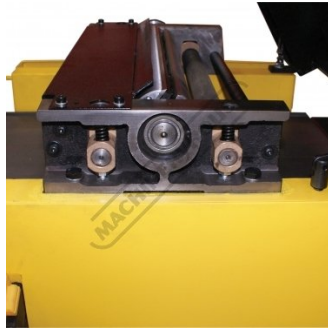
Solid Cast Bearing Supports
