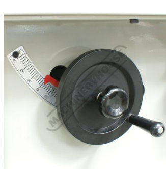
Blade Height Adjustment Handle and Angle Scale
