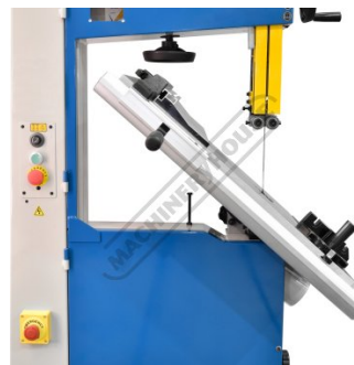
Cast Iron Table Tilts to 45 Degrees
