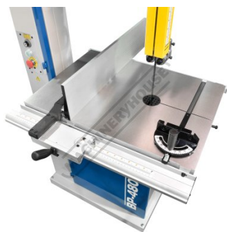
Large Cast Iron Table and Mitre Guide
