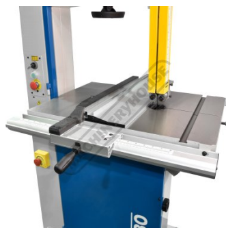
Sliding Rip Fence Down Position
