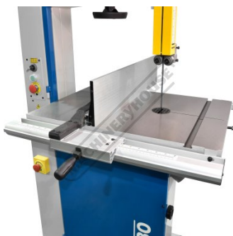
Sliding Rip Fence Up Position
