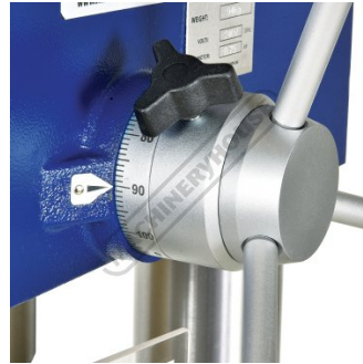
Drill Depth Setting with Scale
