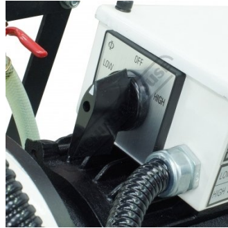
Main Power Switch
