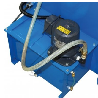
Coolant Pump and Tank
