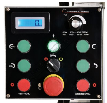
Control Panel With Digital Speed Readout
