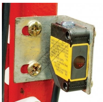
Safety Omron E32S Rear Light Sensor Guarding
