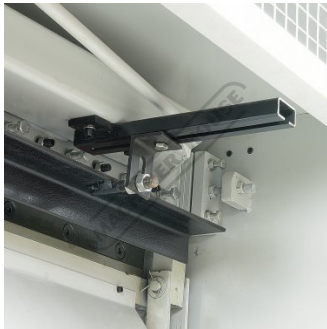
Backgauge Close Up
