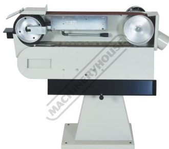
Side Open for Belt Replacement
