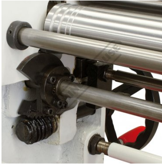
Rear Curving Roller Cam Mechanism
