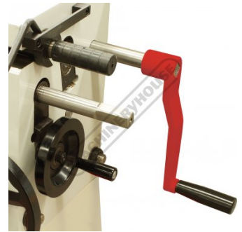
Low Speed 3.5 to 1 Drive Handle Position
