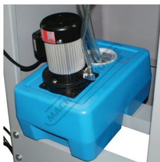
Coolant Pump and Tank
