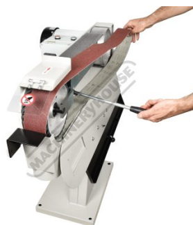
Quick Release Belt Replacement
