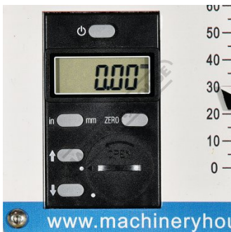
Digital Readout on Quill Depth
