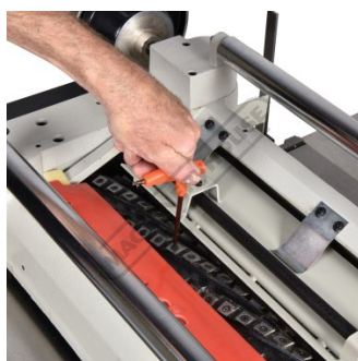
Six Spiral Cutter Head Changing Insert
