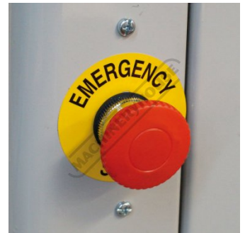
Raised Emergency Stop
