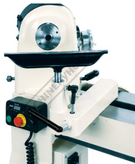
Swivel Headstock with Spindle Lock and Indexing
