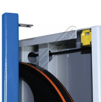
Safety Micro Switch On Door
