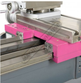
Slides Ready For Mounting of DRO Scales
