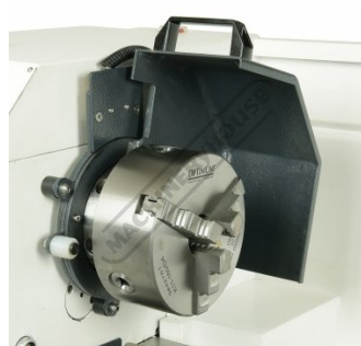
Safety Chuck Guard Open Position
