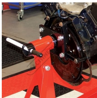
Mounting Position Shown with Ford 351 Engine
