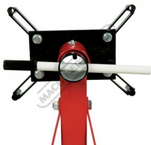
Index Lock Pin In Position 5
