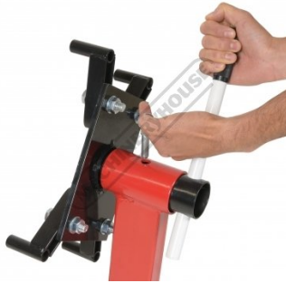
Index Lock Pin Released For Rotating
