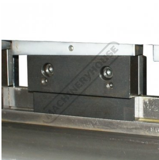
Adjustable Top Tool Taper Wedge System
