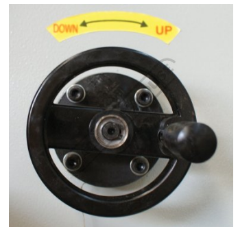
Fine Adjustment Beam Positioning
