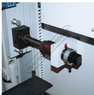
Quick Action Blade Clearance Adjustment
