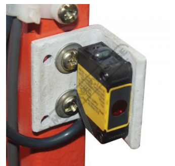
Safety Omron E3ZS Rear Light Sensor Guarding
