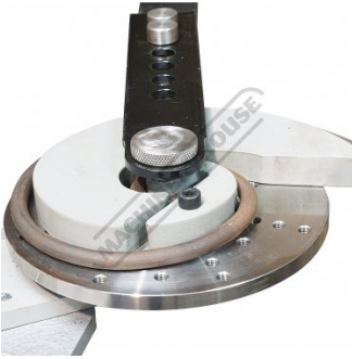
Shown Bending Round Bar Scroll
