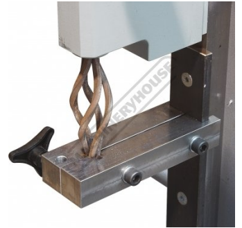
Shown Twisting Multiple Bars
