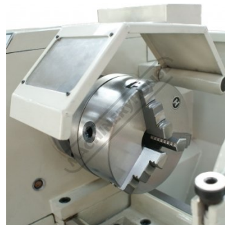
Chuck Guard With Safety Micro Switch
