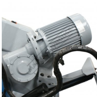
Motor and Gearbox Drive
