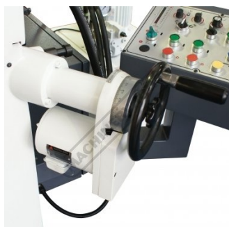
Fine Feed Height Adjustment Dial
