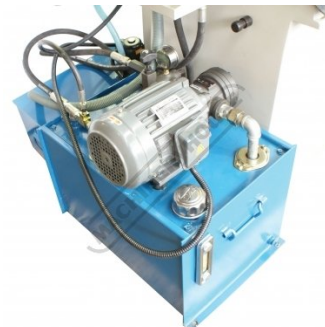
Hydraulic Unit & Coolant Tank
