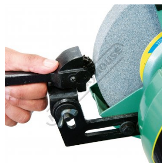
Setup for Dressing a Grinding Wheel Close Up
