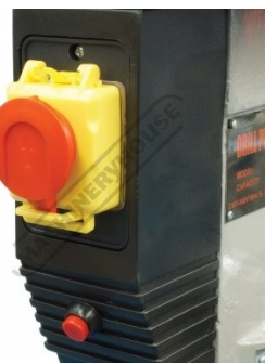
Emergency Stop Switch and Light Switch
