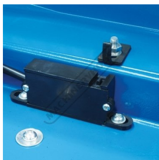
Safety Micro Switch on Pulley Guard
