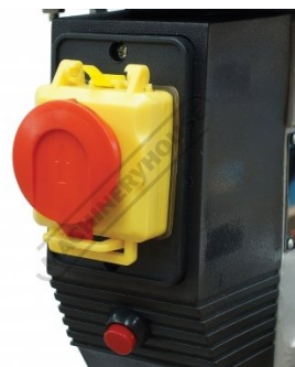
Emergency Stop Emergency Switch and Light Switch
