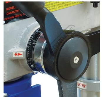
Drilling Depth Stop Setting With Scale
