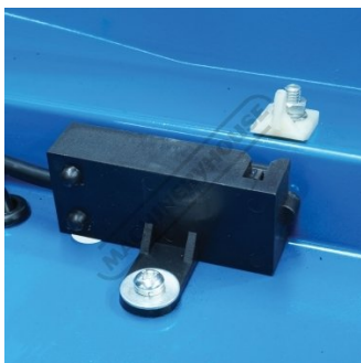
Safety Micro Switch on Pulley Guard
