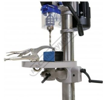
Shown Clamping Job on Drilling Machine Low View
